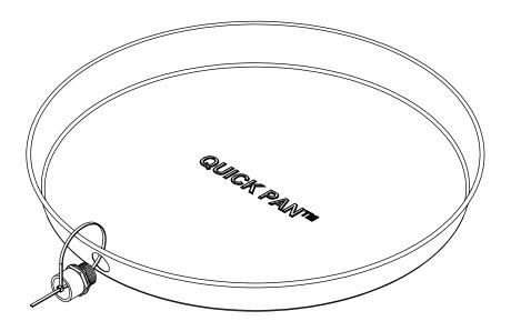
The HOLDRITE® QUICK PAN™ provides a quick simple solution when a drain pan is required under a water heater. These pans are suitable for both electric and gas water heaters. Available in five sizes (20" - 28"). Model #QP-20 (20"), #QP-22 (22"), #QP-24 (24"), #QP-26 (26") and #QP-28 (28"). Pan depth is 2-1/2".
